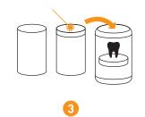
Releasing of the build platform, sliding it inside the recovery cylinder; positioning of the new build platform, starting of the next printing cycle.
