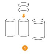
Positioning of the build platforms in the work cylinder.
